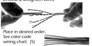
3. Trim wire ends so all conductors are equal length and uniform. Use built in wire cutter in EZ-RJ45® Crimp Tool.
